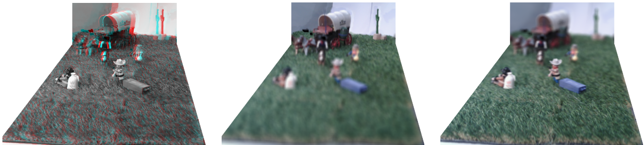
Figure 1: Virtual stereo pair with user-adjustable inter-axial distance (left), synthetic aperture renderings (center, right)
